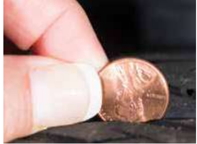
If you can see the top of Lincoln’s head, it’s time for new tires.
